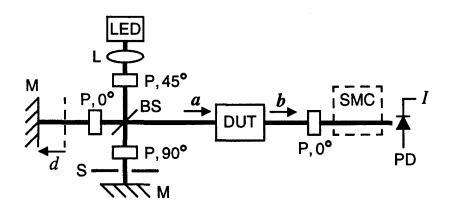
**Figure 1.** Apparatus used for measurement of polarization mode dispersion using frequency scanning and interferometry. LED: light emitting diode; L: lens; P: linear polarizer; BS: beamsplitter; M: mirror; DUT: device under test; SMC: scanning monochromator; PD: photodiode.
