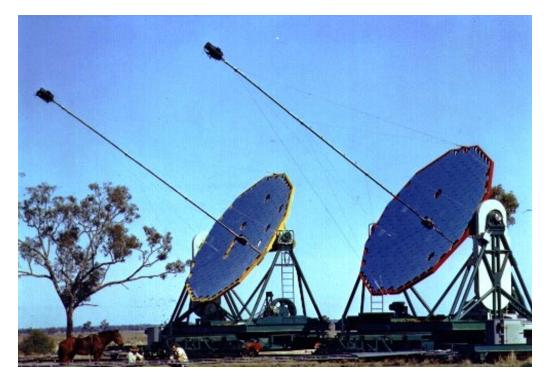
**Fig.3.** The only previous astronomical instrument which could have segregated among the light sources of Fig. 1. The original *intensity interferometer* at Narrabri, Australia, observed one star simultaneously with two telescopes, whose mutual distance was gradually changed. (University of Sydney; reprinted with permission from its School of Physics)
