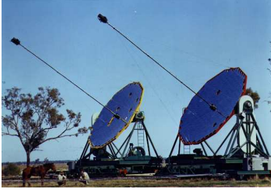
Fig. 2. The two Narrabri Stellar Intensity Interferometer telescopes. Photo from OLBIN (50), courtesy of Prof. John Davis
