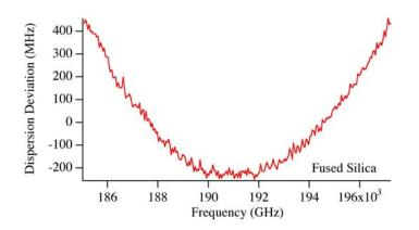
Figure 1 - Measured Dispersion of a Fused Silica Etalon across the C&L Telecom Band
