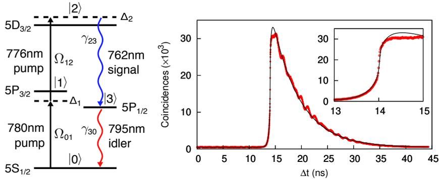
Fig. 1. (Left) Atomic level configuration in a four-wave mixing experiment and time evolution of the population of level  $|3\rangle$ , conditioned on the detection of a signal photon. (Right) Histogram  $G_{\text{FWM}}(\Delta t)$  of detection time differences for photons pairs generated by four-wave mixing in the cold cloud of <sup>87</sup>Rb. The continuous line shows the result of the best fit of the heuristic model. Inset: detail of the sharp rise corresponding to a quantum jump.
