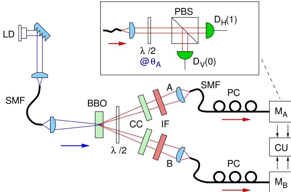
FIG. 1: Schematic of the experimental set-up. Polarization correlations of entangled-photon pairs are measured by the polarization analyzers  $M_A$  and  $M_B$ , each consisting of a half wave plate ( $\lambda/2$ ) followed by a polarization beam splitter (PBS). All photons are detected by Avalanche photodetectors  $D_H$  and  $D_V$ , and registered in a coincidence unit (CU).
