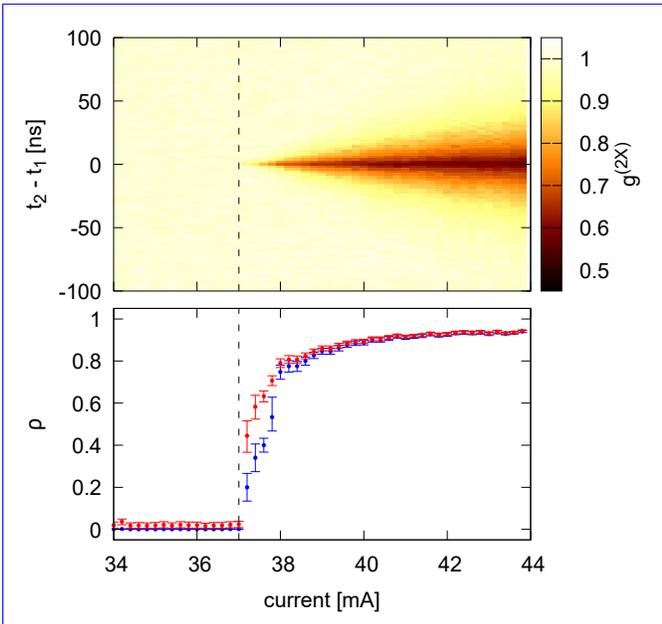
FIG. 4. Top: Interferometric photon correlations  $g^{(2X)}$ , measured for a range of laser currents around the lasing threshold. Bottom: Corresponding upper bound of fraction  $\rho$  of coherent light (red) extracted via Eqn. 13, and the lower bound (blue) extracted via Eqn. ??-14 from  $g^{(2X)}(0)$ . The dotted line indicates the lasing threshold of 36.437 mA.
