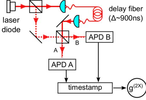
FIG. 1. Experimental setup for measuring interferometric photon correlations. Light from a laser diode enters an asymmetric Mach-Zehnder Interferometer. Single photon avalanche photodetectors (APD) generate photodetection events at each output port of the interferometer, which are time-stamped to extract the correlations numerically.
