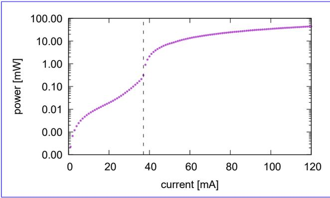
FIG. 3. Purple circles: power against current measurement of the laser diode, taken from 1 to 120 mA in steps of 1 mA. The sharpest change in current was measured at 37 mA, shown in dotted lines.
