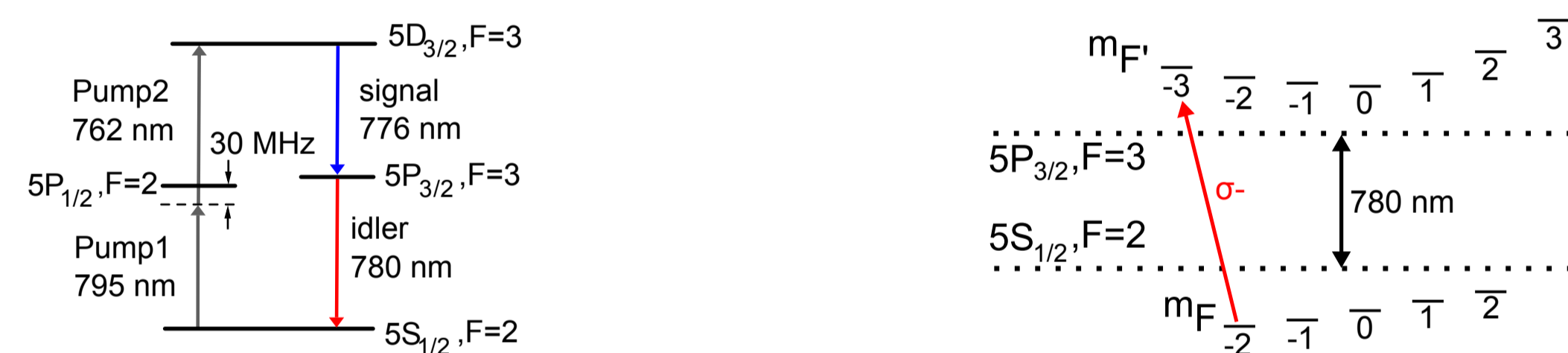
FIGURE 1: Energy level schemes of 87 Rb showing the cascade decay scheme of the FWM process (left) and the closed transition along which the single atom is excited and spontaneously emits a single photon (right).
