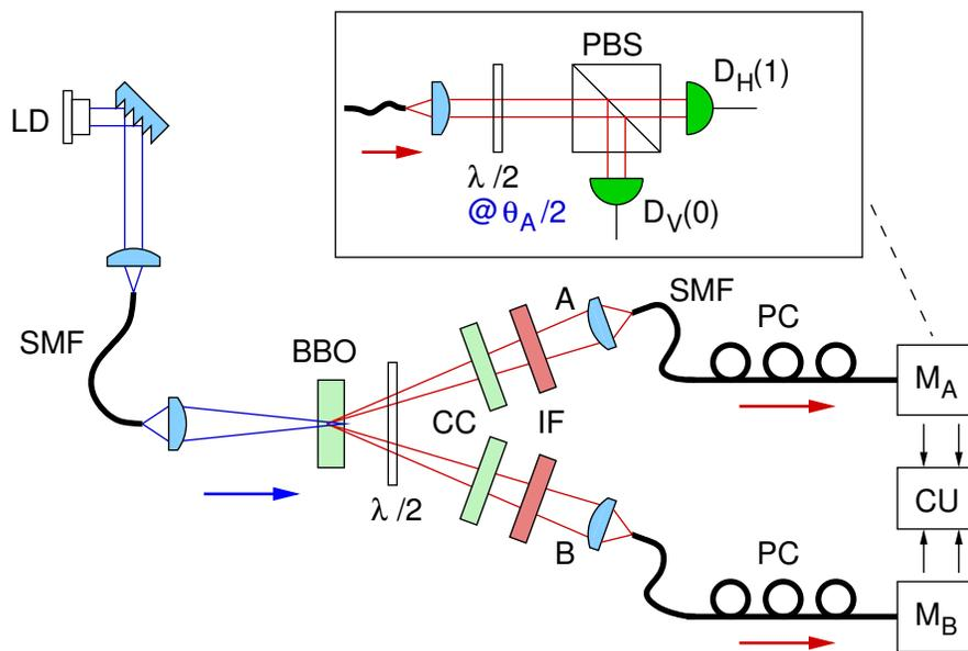
**Figure 5.** Schematic of the experimental set-up. Polarization correlations of entangled-photon pairs are measured by the polarization analyzers  $M_A$  and  $M_B$ , each consisting of a half wave plate ( $\lambda/2$ ) followed by a polarization beam splitter (PBS). All photons are detected by Avalanche photodetectors  $D_H$  and  $D_V$ , and registered in a coincidence unit (CU).
