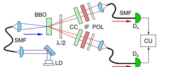
FIG. 2. Schematic of the experimental set-up. Polarization correlations of entangled-photon pairs are measured by film polarizers (POL) placed in front of the collection optics. All photons are detected by silicon avalanche photodetectors  $D_A$  and  $D_B$ , and registered in a coincidence unit (CU).
