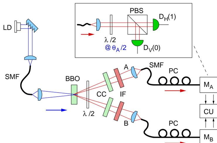
Figure 1: Schematic of the experimental set-up. Polarization correlations of entangled-photon pairs are measured by the polarization analyzers  $M_A$  and  $M_B$ , each consisting of a half wave plate ( $\lambda/2$ ) followed by a polarization beam splitter (PBS). All photons are detected by Avalanche photodetectors  $D_H$  and  $D_V$ , and registered in a coincidence unit (CU).
