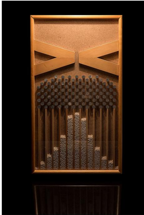
Fig. 1.1 The bean machine, also known as the Galton Board, invented by Sir Francis Galton [35]. The copyright of the image belong to [36]. Beans are dropped from the top. For an individual bean, when it hits the pegs, it either bounces left or right. Finally it will end at one bin at the bottom.
