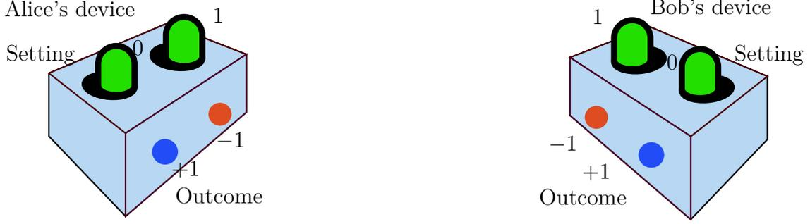
Fig. 1.3 A simplified CHSH Scheme. Alice and Bob each have a measurement device with two settings  $x, y \in \{0, 1\}$  and two outputs  $a, b \in \{-1, 1\}$ . Bell tests are carried out in successions of rounds. Each party chooses a measurement setting and records the measurement outcome in every round.
