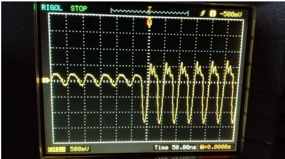
Figure 12. Signal output after passing through the FM board. Sinusoidal signal seems to be distorted.
