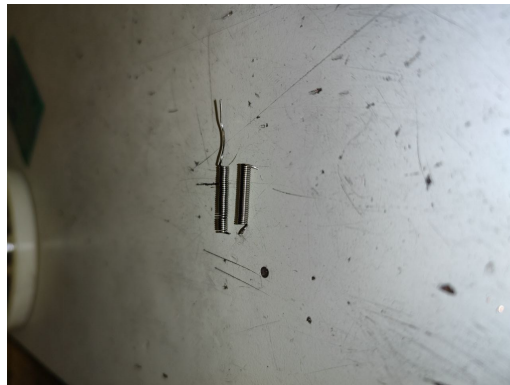
(f) Cut spring down to length and to avoid kinks
