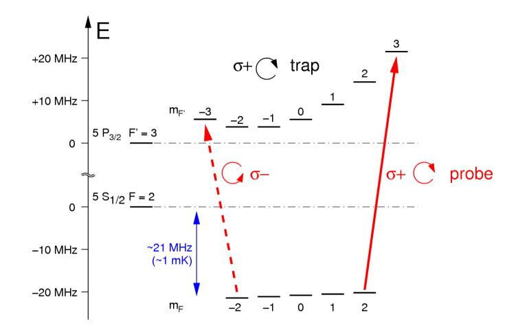
optically pump with the probe beam into 2-level system
