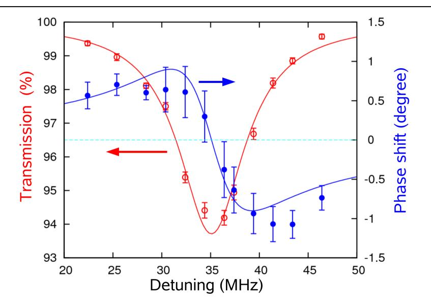
phase shift within factor 2..3 of prediction by stationary atom model!
