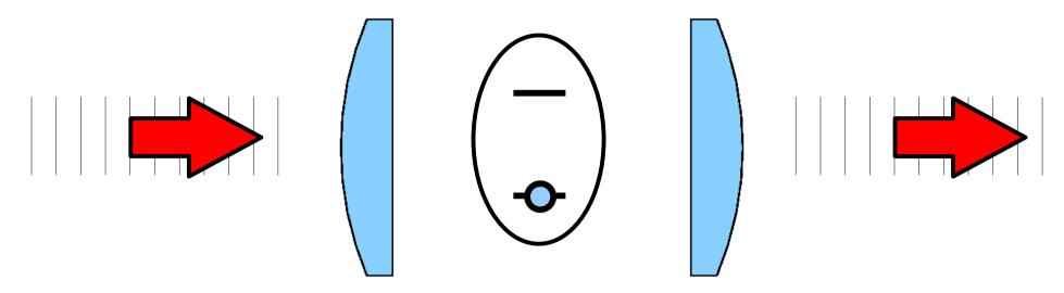
• use a **focusing lens pair** to enhance center mode function:
